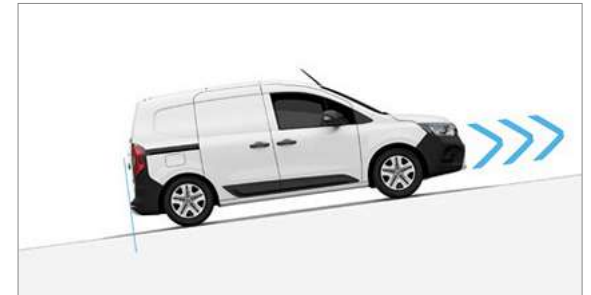
hill start assist. Combined with ESC, hill start assist maintains brake pressure automatically for 2 seconds to give you time to lift your foot from the brake pedal and press the accelerator. The system activates when the slope exceeds 3%. Available as standard on all models.
